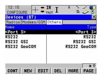
7. Press F3 for edit. Use the arrow keys to set the communication parameters to match the image below.
